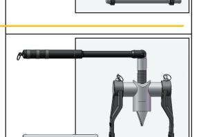
**3.** To Remove the left hand cast leg from the tool. Pull the spring loaded plunger to release the
