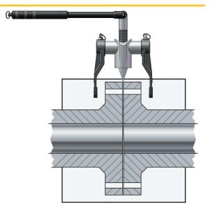
**4.** Engage the spreading bar through the leg of the tool and the flange stud hole.
